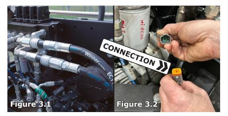
The two quick-connect hose fittings (Figure 3.1) and the cooling electrical connection (Figure 3.2) can only be plugged in a certain way. This is to prevent improper use and makes attachments quick and easy to install.
