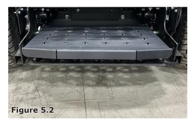
The Force has a new safety feature called an Operator Presence Switch, which is built into the Force platform. If the operator leaves the platform, the switch will put all Force attachments into Fault Mode and will not function until the operator stands on the platform and resets the toggle switch.
