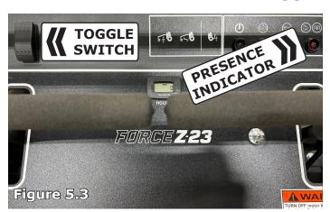
The toggle switch has three positions: Forward, neutral and reverse. The AERA-Vator doesn't use the reverse function. If the AERA-Vator goes into Fault Mode the Presence Indicator light will flash until reset.
